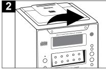
Press the CD OPEN/CLOSE button to open the CD compartment door.
